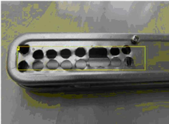
1. Drill holes for LEDs
