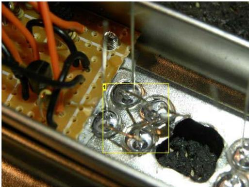
1. Solder Anodes to Cathodes of LEDs
