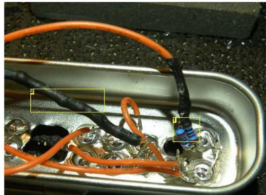
1. Soldered LEDs to resistors
