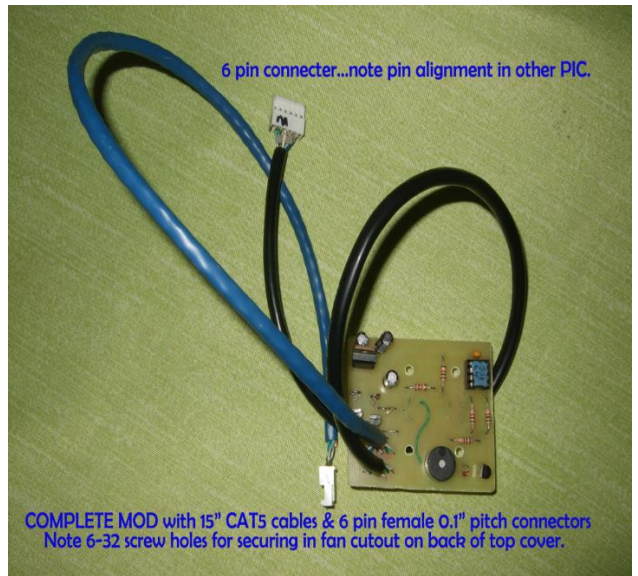
FRONT BLCK CAT 5 to RELAY BRD HDR on BASE INSIDE OF APACHE COVER STOCK LED DISPLAY ADD On MOD BLUE CAT 5 to 6 pin DISPLAY HDR REAR
