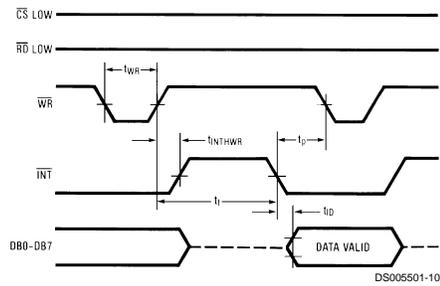
FIGURE 5. WR-RD Mode (Pin 7 is High)
