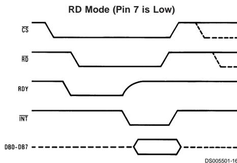
When in RD mode, the comparator phases are internally triggered. At the falling edge of  $\overline{RD}$ , the MS flash converter goes from zero to compare mode and the LS ADC's comparators enter their zero cycle. After 800 ns, data from the MS flash is latched and the LS flash ADC enters compare mode. Following another 800 ns, the lower 4 bits are recovered.
