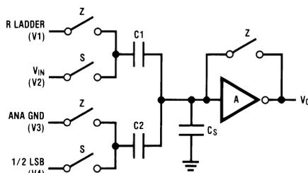
FIGURE 8. ADC0820 Comparator (from MS Flash ADC)
