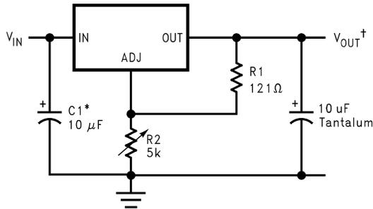
\*NEEDED IF DEVICE IS FAR FROM FILTER CAPACITORS
