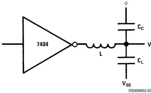
**FIGURE 5. Clock Coupling**
