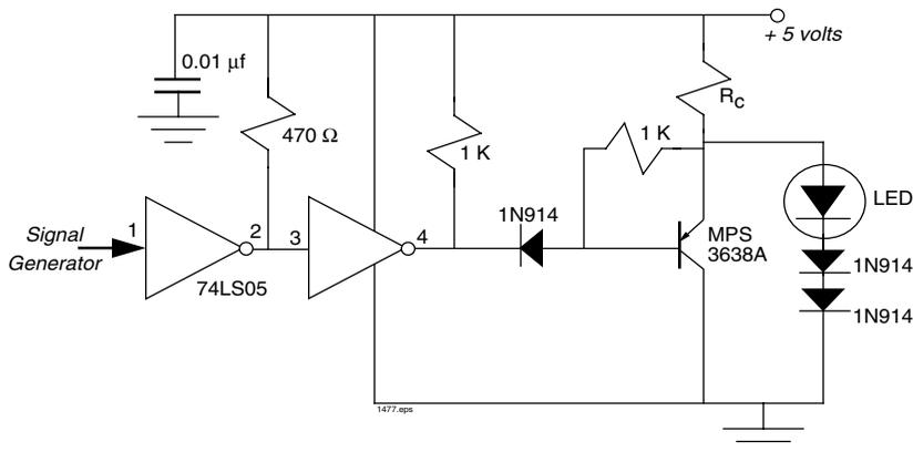
**Figure 8.5** Ten-megabit push-pull LED drive circuit.
