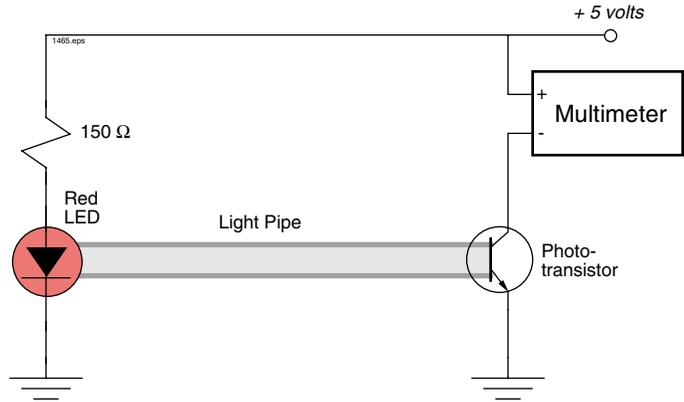
**Figure 2.2 Test circuits for evaluating light guide.**
