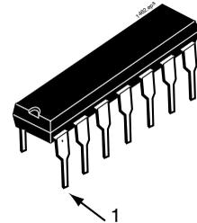
**Figure 1.3 A 14-pin integrated circuit (IC) in a dual-in-line-package (DIP).**
