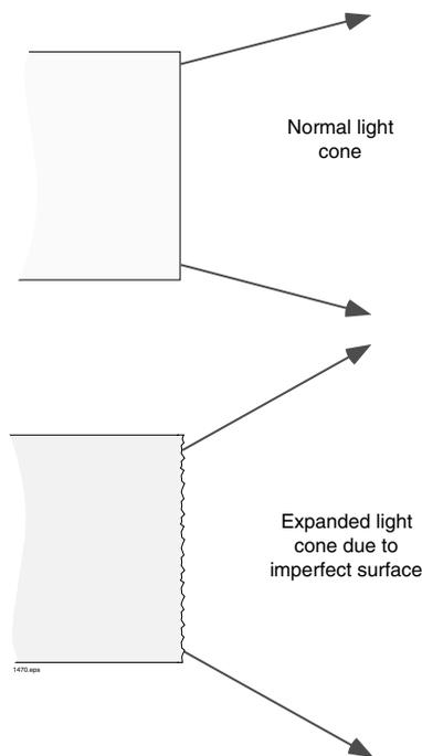
**Figure 6.1** (Top) Fiber with a perfectly flat termination, arrows depicting the cone of light exiting the fiber core. (Bottom) A poor fiber polish/termination showing the resultant increased divergence of exiting light rays.
