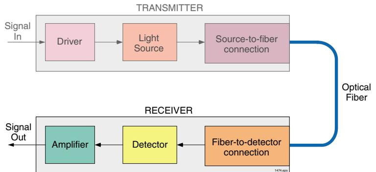
**Figure 9.1** Basic elements found in a fiber optic link with the receiver amplifier portions highlighted.
