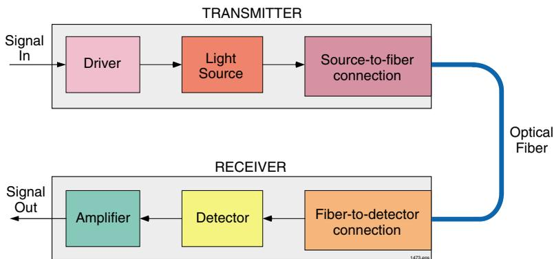
**Figure 8.1** Basic elements in fiber optic links.
