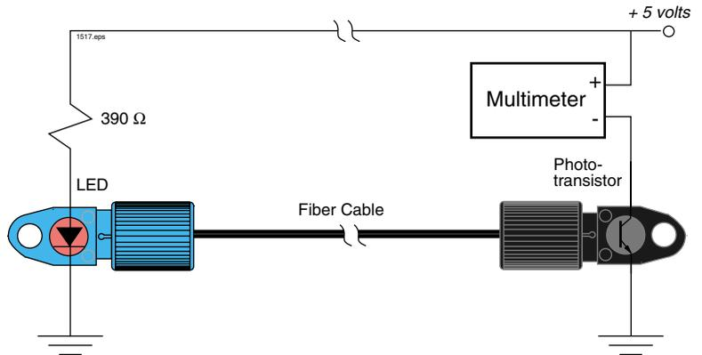
**Figure 3.2** Test circuit for measuring cable transmission.
