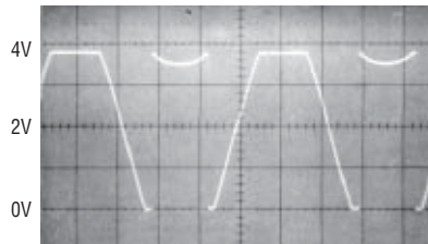
LM324, LM358, OP-20 EXHIBIT OUTPUT PHASE REVERSAL
