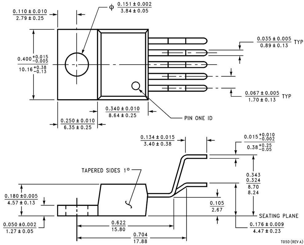
**5-Lead TO-220 Bent and Staggered Package**
