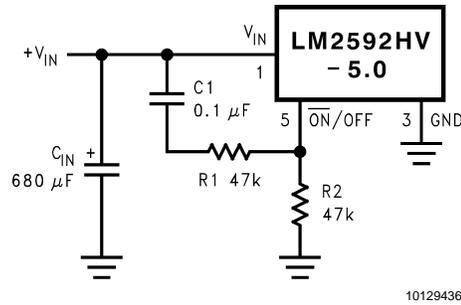
FIGURE 7. Delayed Startup
