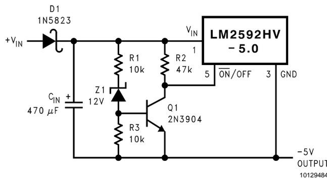
This circuit has an ON/OFF threshold of approximately 13V.
