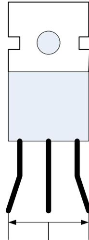
Recommended lead spread for voltage regulator. For datasheets of part number 23579 (LM317T) and 23819 (LM337T) please proceed to our website at [www.jameco.com](http://www.jameco.com)
