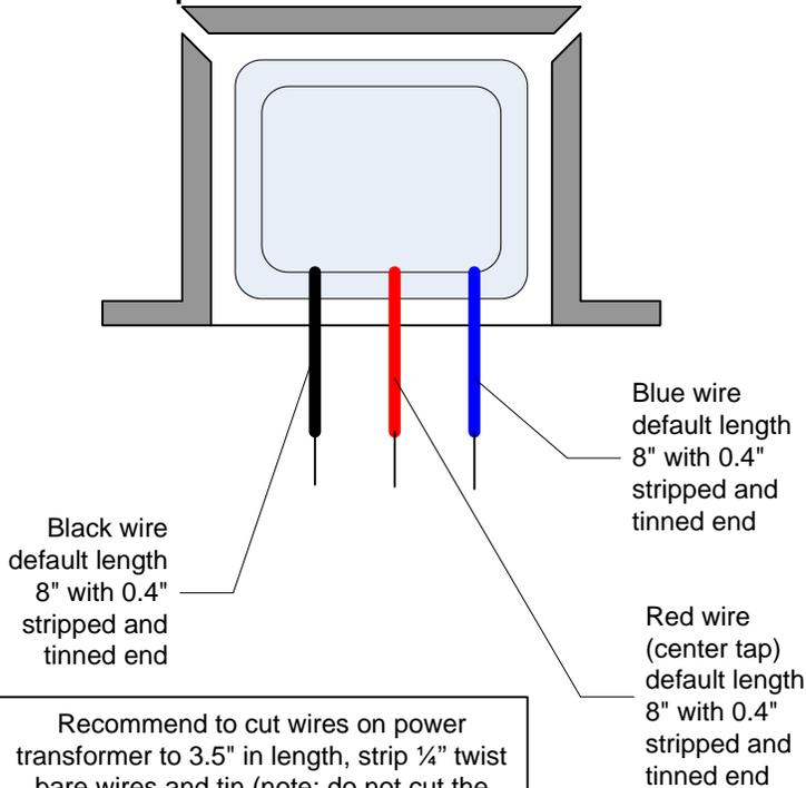
Recommend to cut wires on power transformer to 3.5" in length, strip ¼" twist bare wires and tin (note: do not cut the wires while stripping)
