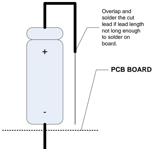
Note: extension lead not required if lead of one end of capacitor is long enough to solder on the board.
