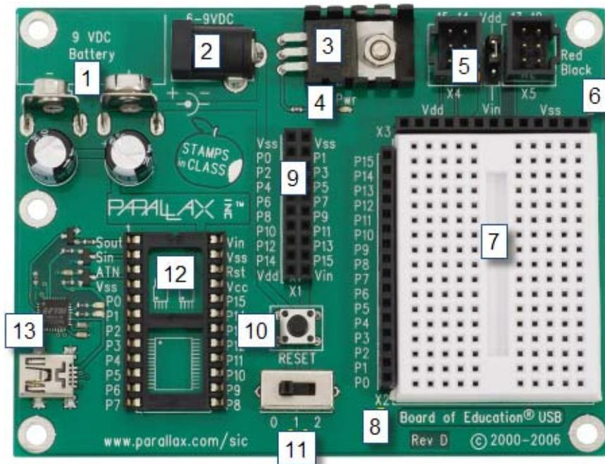
1. **9V Battery Clip:** You can use alkaline or rechargeable 9 volt batteries. The battery clip and barrel jack are intentionally positioned so you cannot use both at once.
