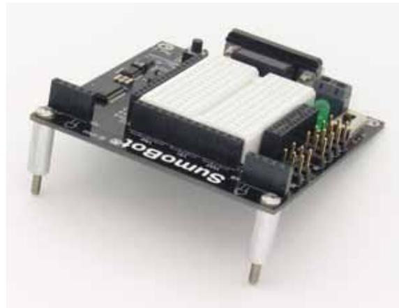
Using a 4/40 1" pan-head machine screw, attach each standoff to the front mounting holes of the SumoBot PCB.
