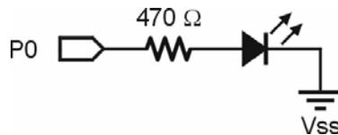
**Figure 3.4: Start LED Connections on the SumoBot PCB**
