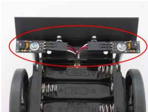
Using two 4/40 1/4" pan-head machine screws, attach the QTI line sensors to the 1-1/4" round stand-offs. Connect the ends of the 10" 3-pin extension cables to the QTI line sensors, noting the polarity markings B[lack]-R[ed]-W[hite] on the QTI sensors.
