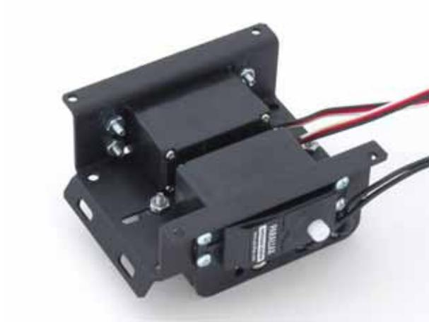
Using four 4/40 3/8" pan-head machine screws and 4/40 nuts, attach each servo motor to the chassis. The easiest way to do this is to hold the nut with one finger while turning the screwdriver with the other hand.
