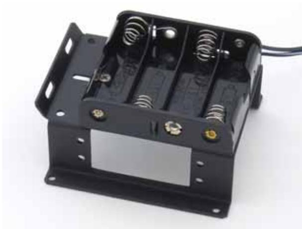
Stand the SumoBot on its PCB mounting ears. Install the plastic battery pack using two 4/40 3/8" flat-head screws and nuts. The screws will be countersunk into the battery pack when tightened and should be out of the way of the batteries.
