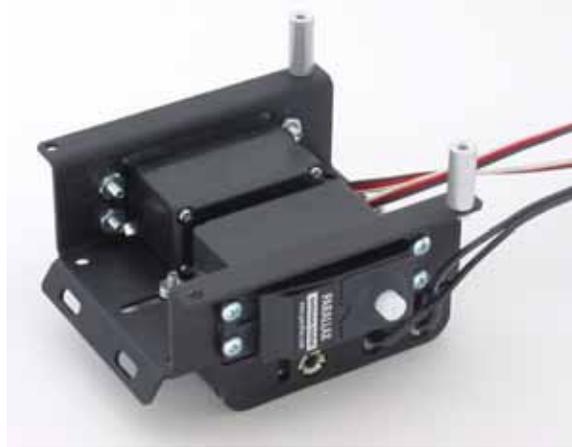
Using a 4/40 3/8" pan-head machine screw, attach each stand-off to the rear of the SumoBot chassis.
