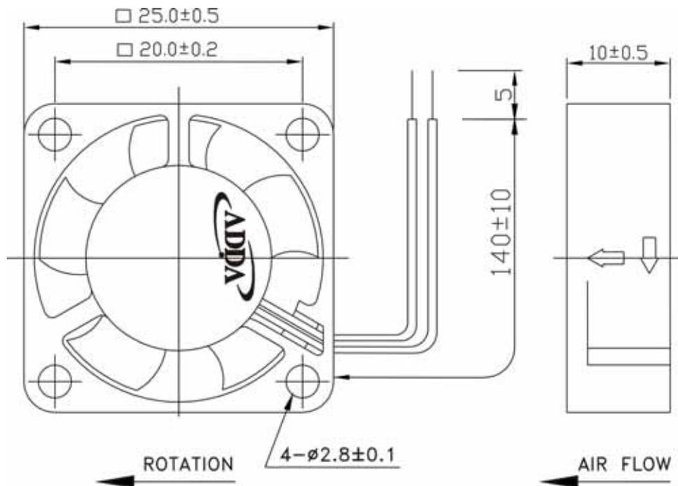
LEAD WIRES : UL 1571, AWG28, L = 140 +/- 10 mm
