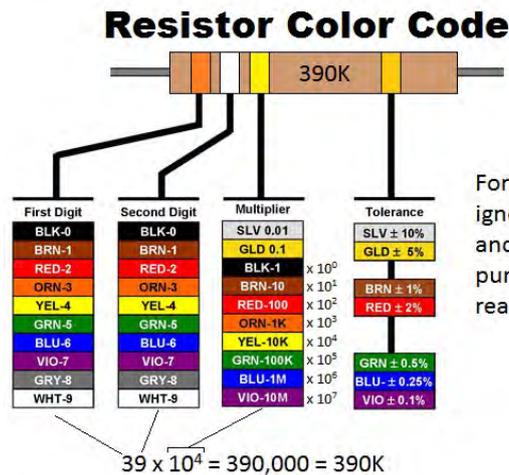
For our purpose, we can ignore the tolerance strip and use it solely for the purpose of orientation for reading the color code.
