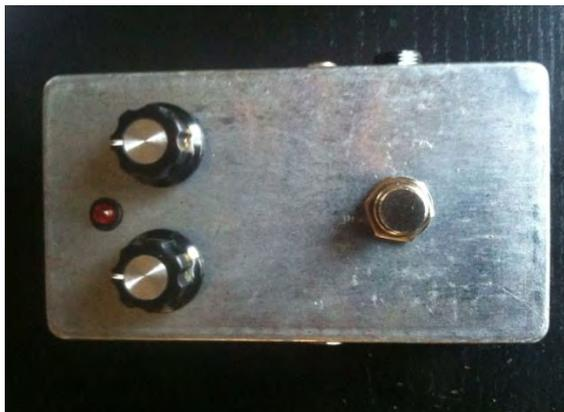
A solid-state overdrive/distortion effects pedal for guitar and other musical instruments. By including or leaving out optional components (included) this pedal can be "tweaked" by you, the builder, during assembly to deliver tones for blues or rock. Or try your own parts to build an effect that is uniquely your own!
