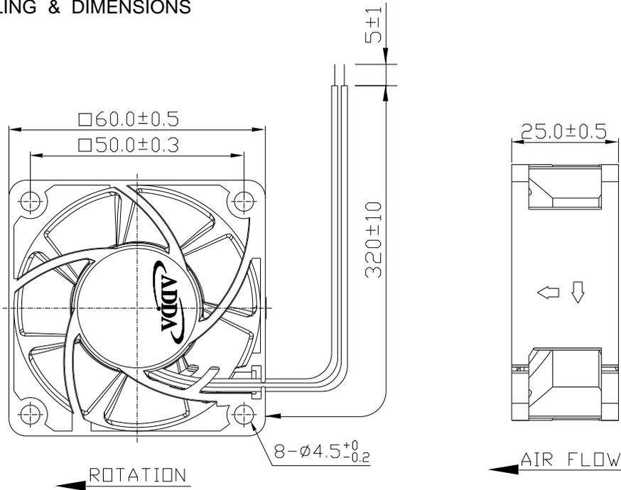
LEAD WIRES : UL 1061, AWG26 , L = 320 +/- 10 mm
