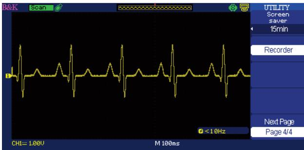
Monitor and analyze long-term signal behavior by recording data continuously over an extensive period of time and playing it back for post acquisition analysis. Data is recorded in a sequence of up to 2500 frames.
