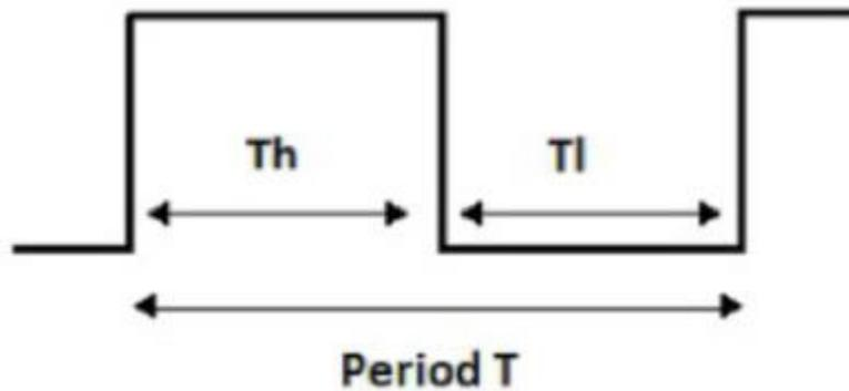
Figure 9: Astable square wave one complete cycle.
