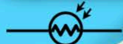
PHOTOCELL (Light Dependent Resistor)
