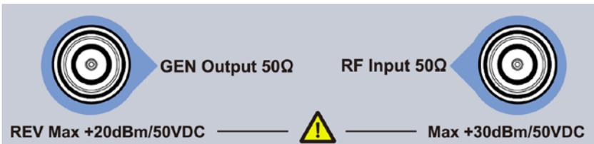
The output of the tracking generator can be connected to a receiver through an N type male connector, users can purchase this option if required.
