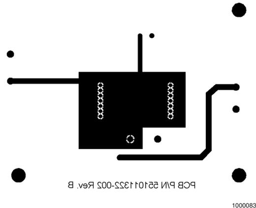
FIGURE 4. Recommended LD PC Board Layout: Bottom-Side Layout
