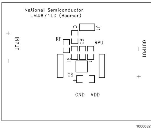
FIGURE 2. Recommended LD PC Board Layout: Component-Side Silkscreen
