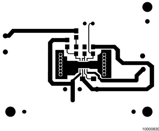
FIGURE 3. Recommended LD PC Board Layout: Component-Side Layout
