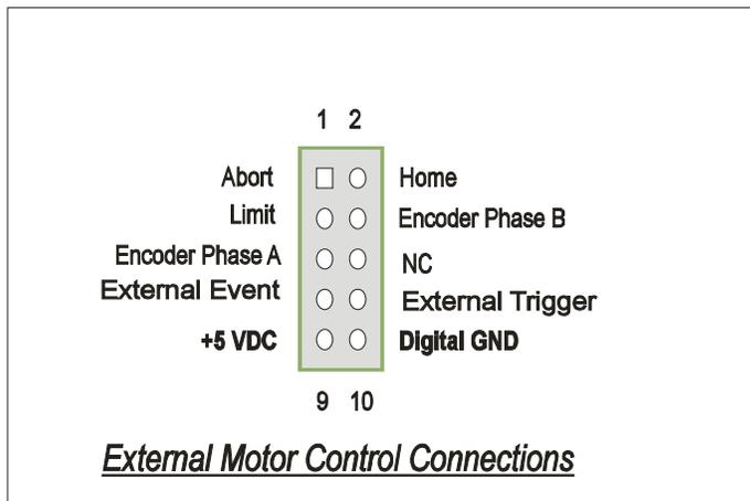
Inputs for home, limit switch and abort are available on the Connector Called “Motor CNTRL”. This 10 pins IDC Connector is showed in Part and Location
