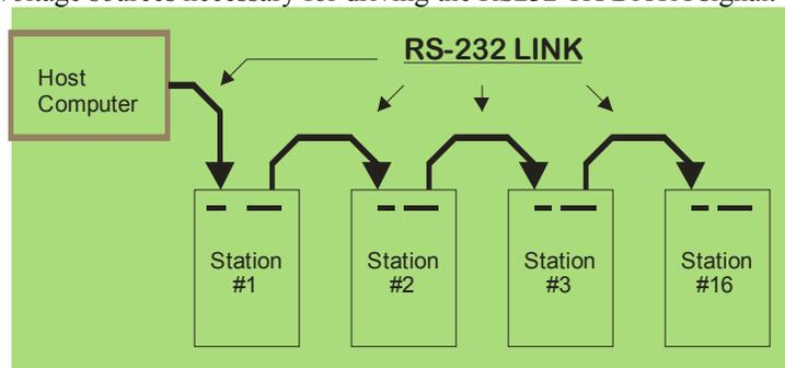
Two driver-receiver pairs handle the RS232 interface. The first one handles communication with the host (or remote board) while the remaining one allows multidrop operation.
