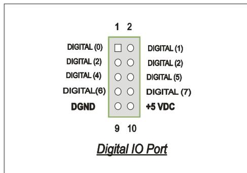
The SPORT232-ST has 8 TTL compatible Input - output lines are available for control of external devices or reading any kind of switches. Each line can sink or source up to 5 mA.
