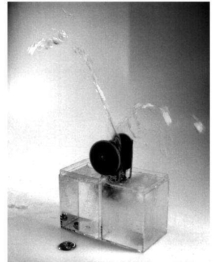
*TiNi Alloy Company's TiNi-I Engine (c 1980) uses a single coil of nitinol wire and can develop speeds of 1000 RPM on just hot and cold water.*
